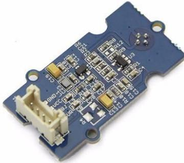
This Grove-Infrared temperature sensor is a non-contact temperature measure model
